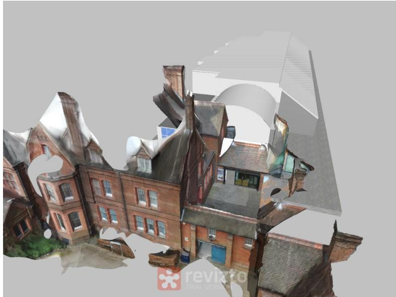
Figure 9: Combined model, incorporating the MERL entrance façade, the inner courtyard (both photogrammetry), and the main galleries (SketchUp)
